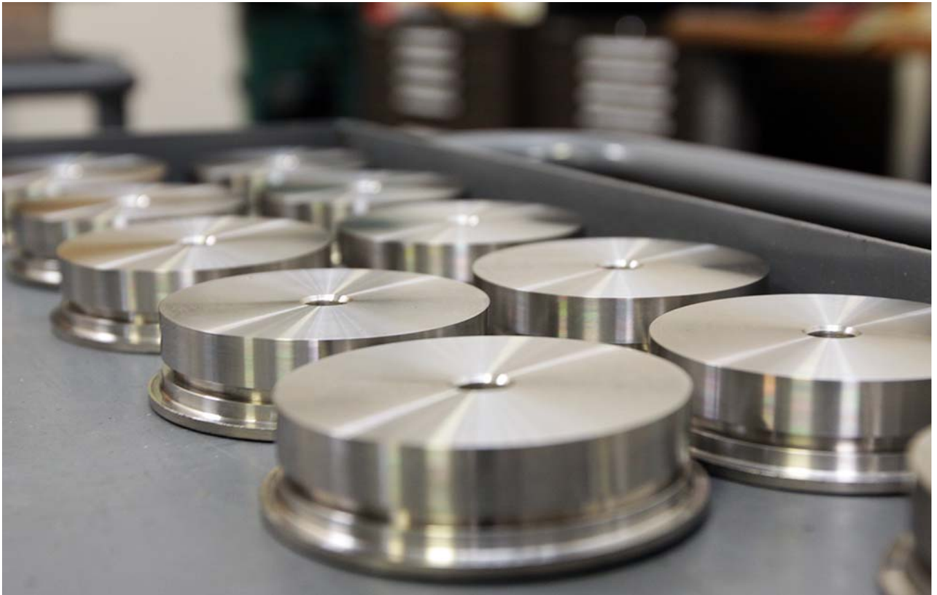
The top portion of the finished Q7 footers.
