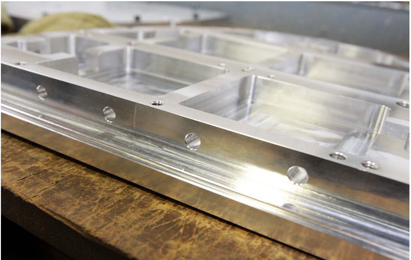
The completed S5 top plate ready for final finishing.
