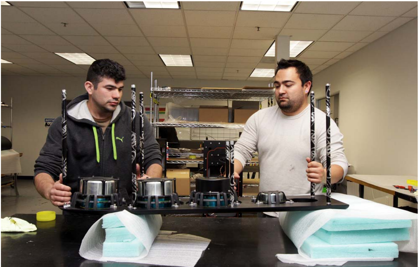
Attaching the front baffle to a Q5 speaker is a two-man job.
