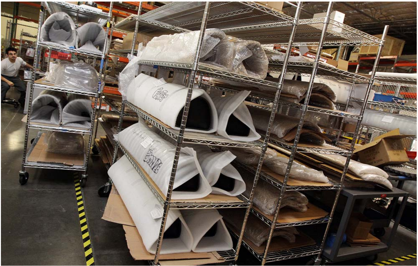
Magico's production process involves working in "rack batches." On this rack are the parts for four pairs of S1 loudspeakers in a variety of finishes.
