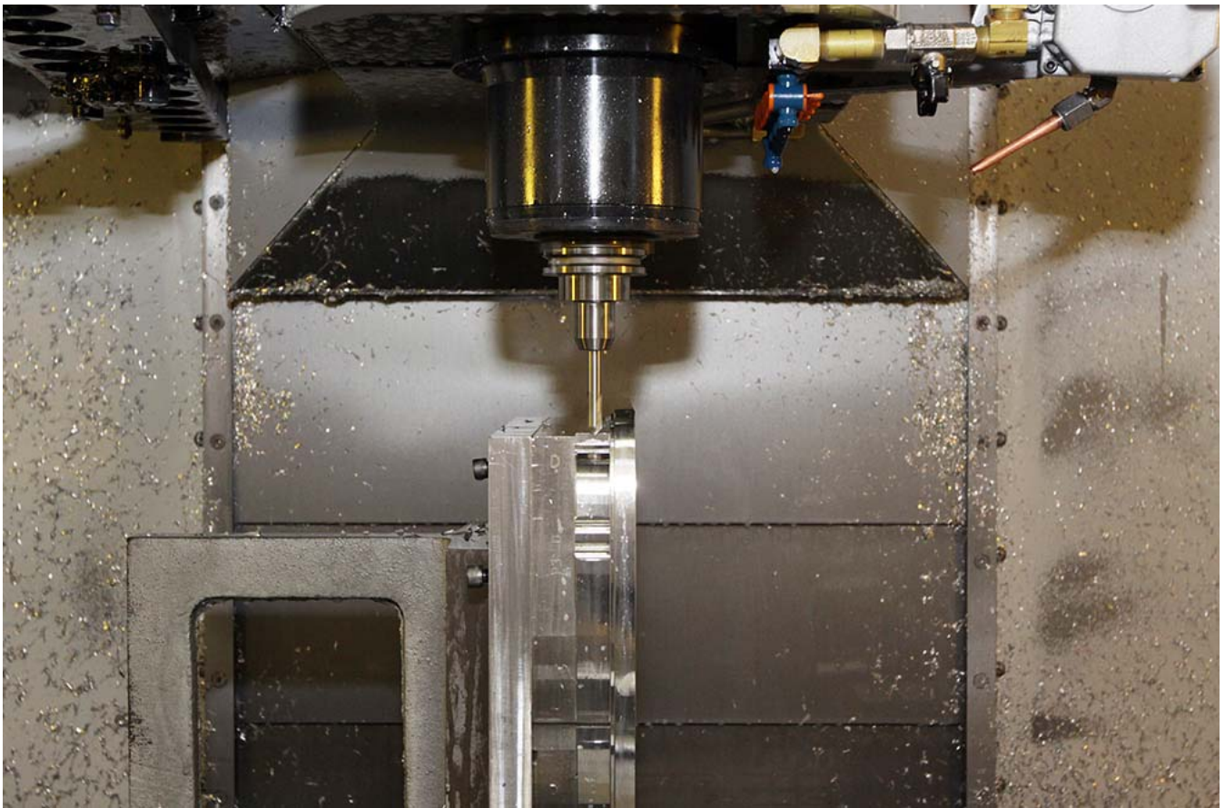
Toward the end of finishing, bolt holes are drilled and then tapped.
