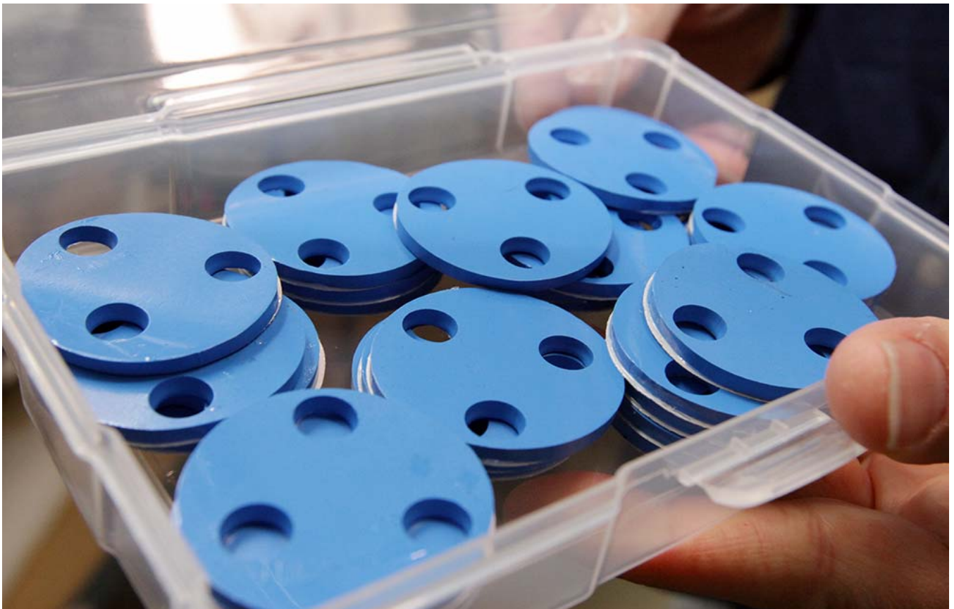
The dampers for the QPod isolators.
