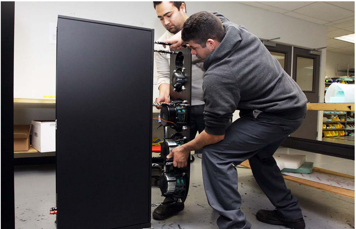
. . . turned vertically and inserted into the metal guide rods that are built into the cabinet.
